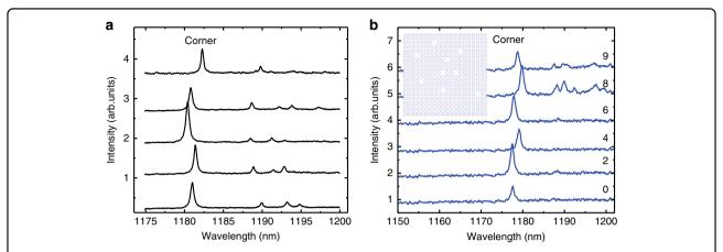
Fig. 3 PL spectra for cavities without and with defects. a PL spectra of defect-free cavities with the parameters of a=380nm, D=242nm and g=50nm. b PL spectra of cavities with different numbers of defects, as shown in the inset. The numbers represent the number of missing square holes in the bulk of the PhC. Here, the missing square holes are several periods away from the corner. The PL spectra are shifted for clarity
